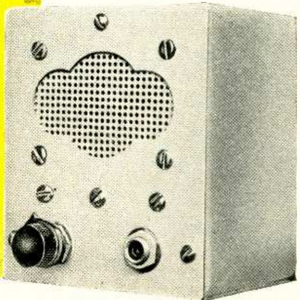
Front view of the miniature transistorized code-practice and a.f. oscillator.
