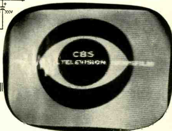
Fig. 2—Insufficient low-voltage supply.
